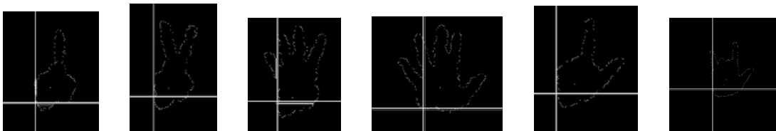
Contour for Hand Gestures 1, 2, 4, 5, 6, 8 respectively. The center point is the cyan point whereas the point of intersection of two lines is the red point.
