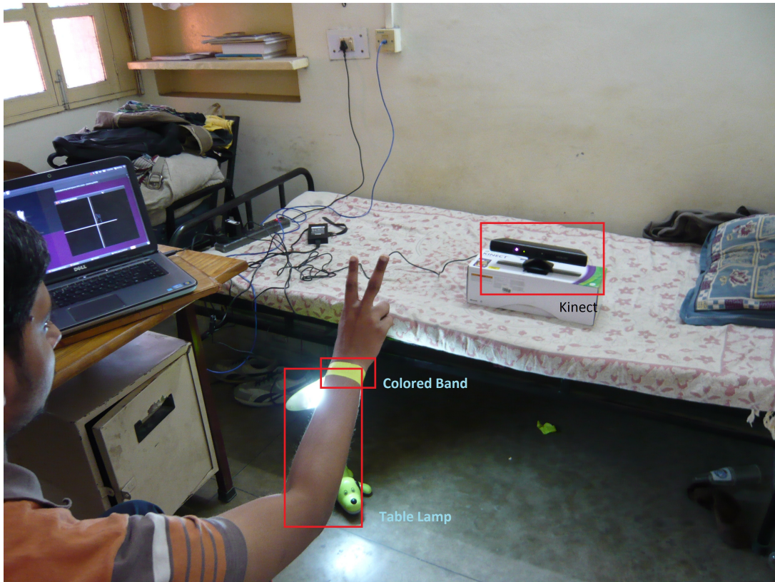
A real time image of the Kinect. The optimum results were obtained at the depth of around 1 meter.
